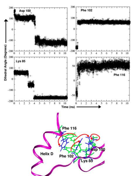
FIGURE 9 Dihedral plots for some key residues that rotate during the dynamics simulation of the ternary complex (simulation 7). In the lower panel the residues are shown before (*green*) and after (*blue*) the dynamics simulation. Dihedral plot for His-115 is not shown, but its flip occurs in the same time range as Phe-116.
